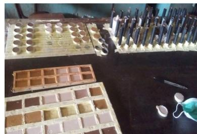
**Figure 2b.** Composites moulds
