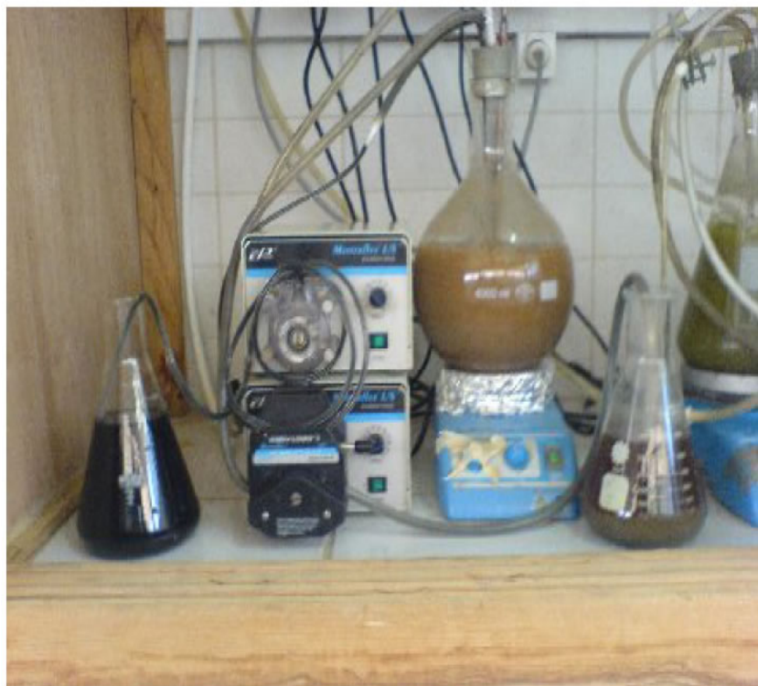
Figure 2. SBR process coupled to the coagulation-flocculation system
