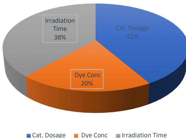
**Figure 5.** Relative importance of input variables to the percentage degradation.
