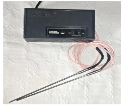
Figure 5: N-Type thermocouples connected to the Sensor-PC module (accuracy: 0.001°C)
