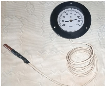
Figure 4: Thermometer used to measure and control the soil temperature (accuracy: 0.5°C)
