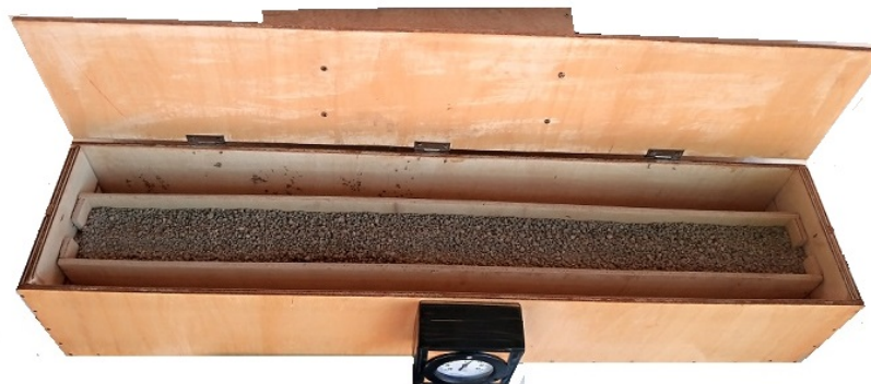
Figure 2b: Interior view of the experimental device filled with cooled soil
