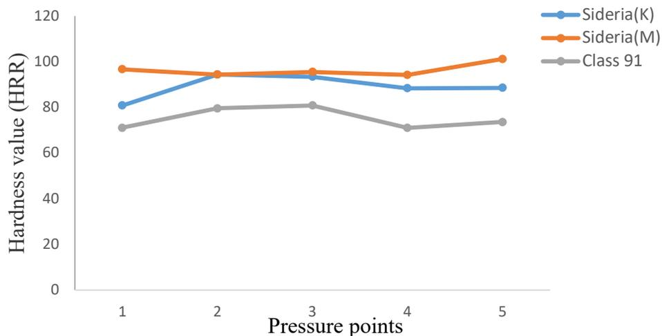
**Figure 5.** Hardness comparison for the three different material samples
