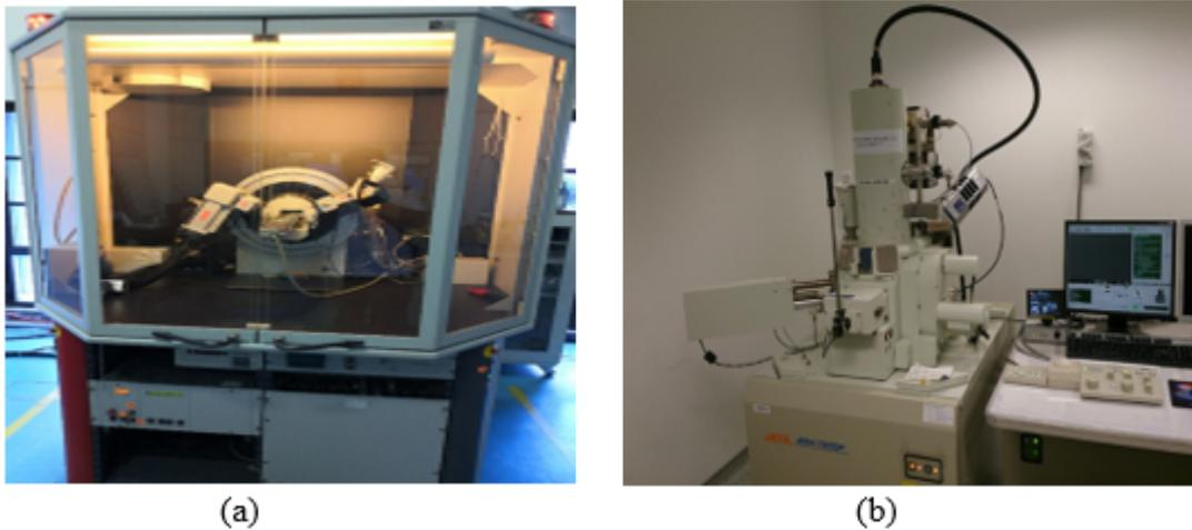
**Figure 4.** Machine for evaluation of sample characteristics for Physical testing for the brake pad samples (a) X-ray diffraction (XRD) machine and (b) Scanning electron microscope (SEM)
