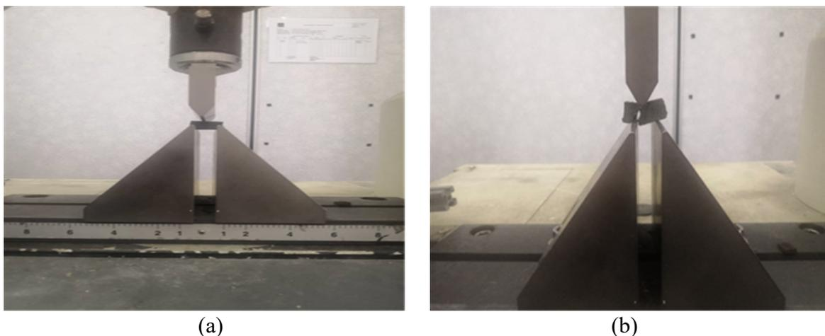
**Figure 6.** The condition of the sample (a) before the transverse rupture strength (TRS) test was performed and (b) after the transverse rupture strength (TRS) test was performed
