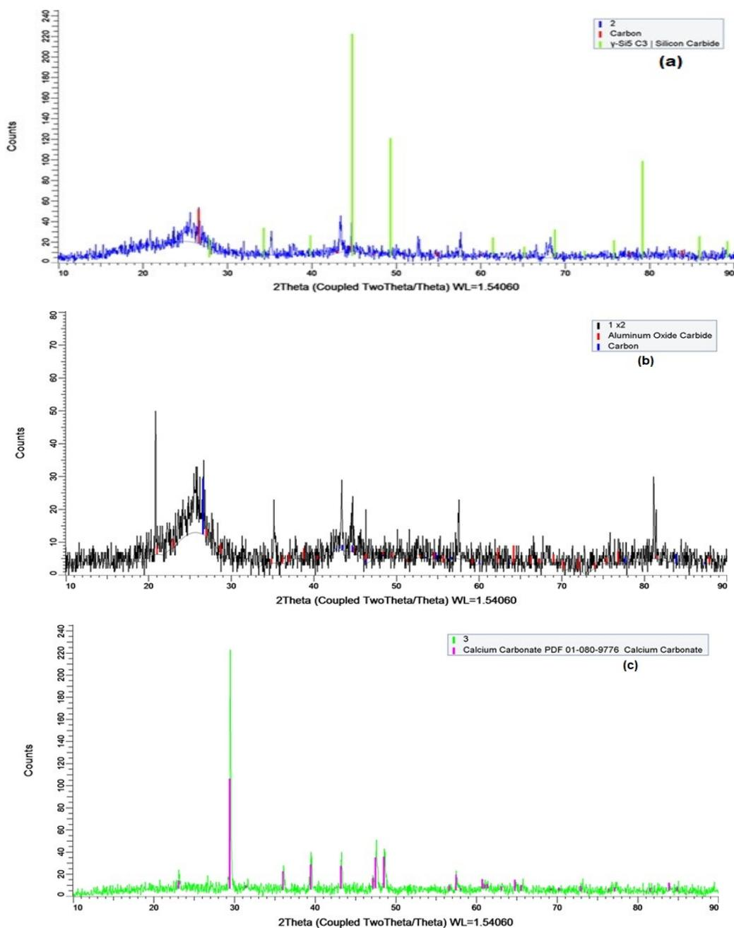
Figure 7. The results of XRD test for the (a) Sideria(K), (b) Sideria(M) and (c) Class91 samples
