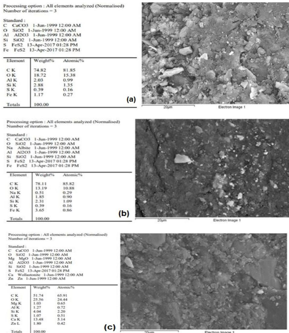
**Figure 8.** The result of the material and topography list for the (a) Sideria(K), (b) Sideria(M) and (c) Class91 samples
