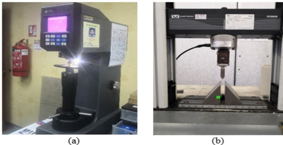
**Figure 3.** Mechanical testing for the brake pad samples (a) Rockwell hardness tester machine and (b) Universal testing machine (TRS)
