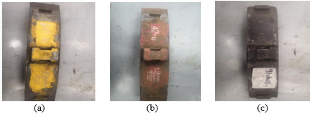
**Figure 2.** Type of materials brake pads tested (a) Sideria(K), (b) Sideria(M) and (c) Class91
