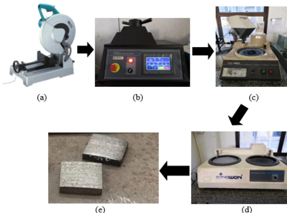
**Figure 1.** Samples preparation processes of brake pad (a) Cutting, (b) Mounting, (c) Scraping, (d) polishing and (e) samples upon completion
