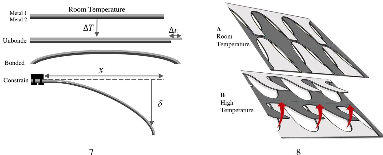
**Figure 7:** Bimetal Strip. Two metals bonded together with different expansion coefficients.
