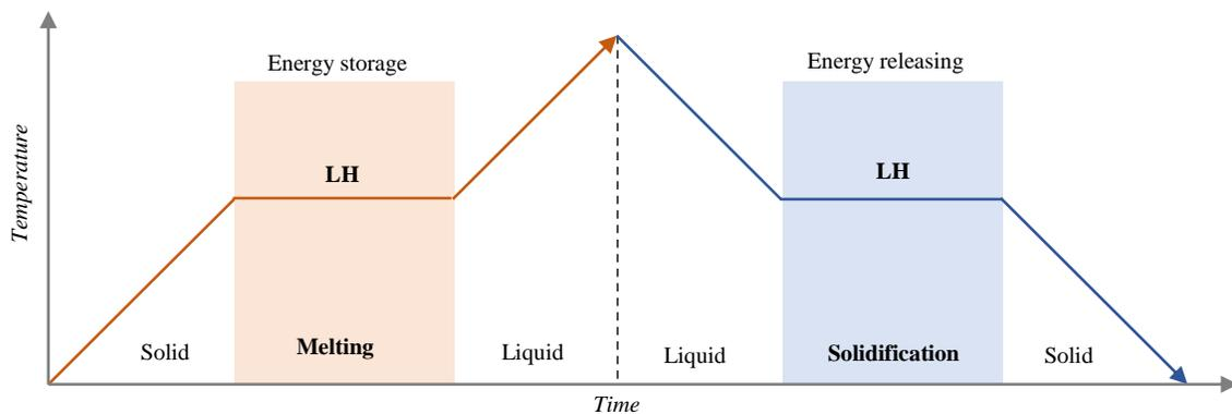
**Figure 14:** Temperature against time PCM behavior. The Latent Heat is stored and released in function of the temperature of the medium, adapted from © Pazrev, 2014 [137].
