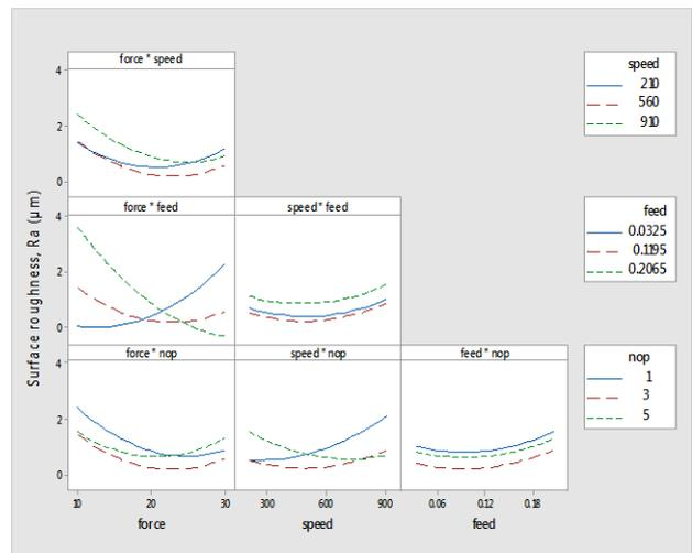
**Figure 4.** Interaction effects of parameters on surface roughness
