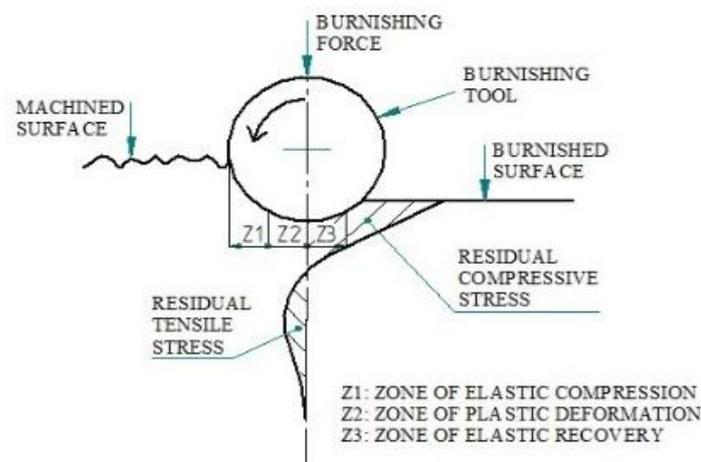
**Figure 1:** Schematic representation of the burnishing process
