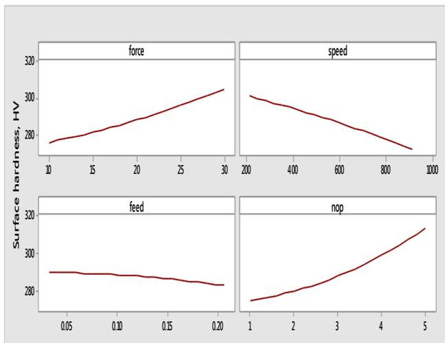
**Figure 5.** Main effect of parameters on surface hardness
