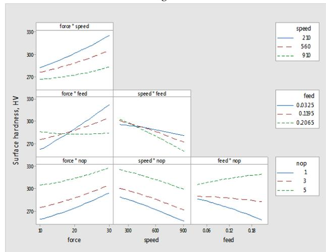
**Figure 6.** Interaction effects of parameters on surface hardness
