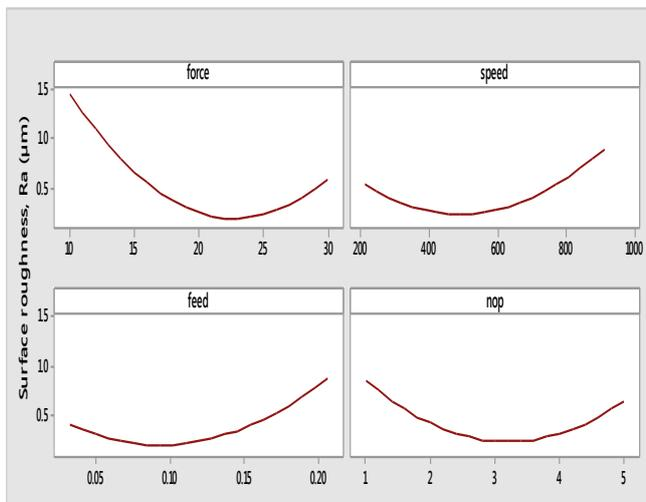
**Figure 3.** Main effects of parameters on surface roughness
