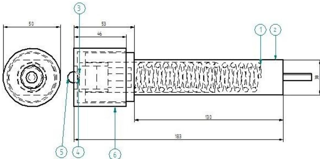
**Figure 2:** Details of the developed ball burnishing tool
