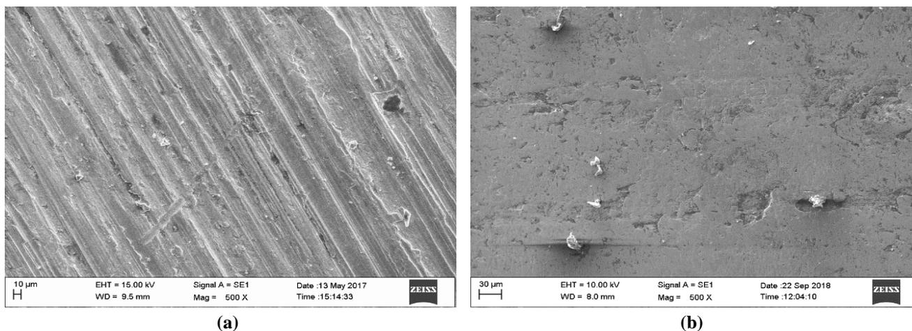
**Figure 7.** SEM images of the turned (a) and burnished (b) specimen
