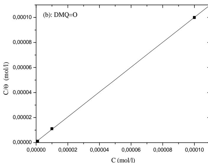
**Figure 10:** Langmuir isotherm adsorption of DMQ=O in 1M HCl from weight loss measurements at 20 °C
