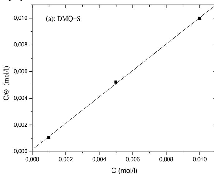
**Figure 9:** Langmuir isotherm adsorption of DMQ=S in 1M HCl from weight loss measurements at 20 °C
