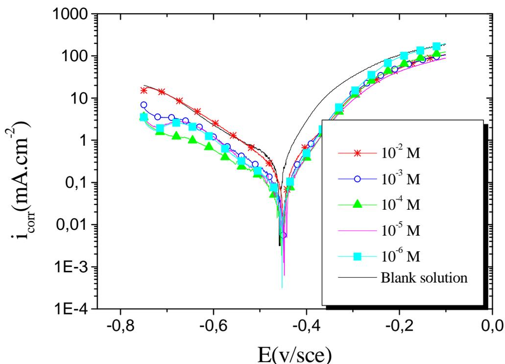
**Figure 3 :** Polarization curves of mild steel recorded in 1M HCl at different concentrations of DMQ=O
