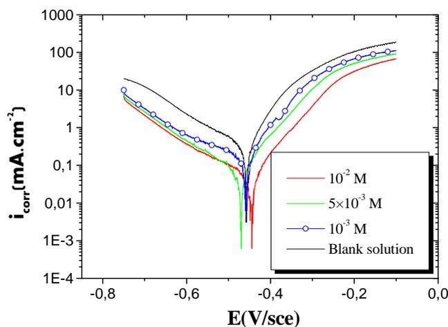
**Figure 2:** Polarization curves of mild steel recorded in 1M HCl at different concentrations of DMQ=S
