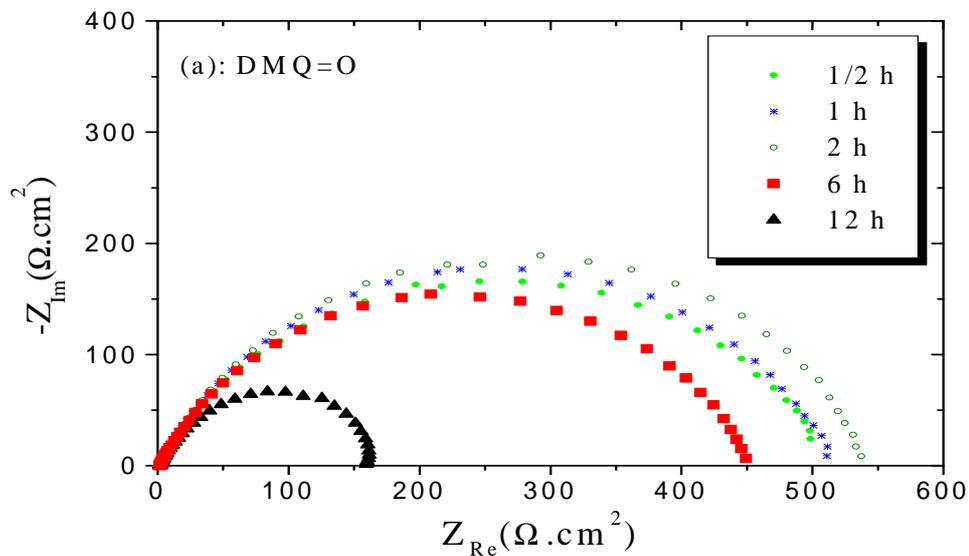
Figure 7 : Nyquist diagrams for mild steel in 1M HCl at different time immersion of  $10^{-4}$  M for DMQ=O
