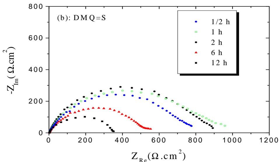
Figure 8 : Nyquist diagrams for mild steel in 1M HCl at different time immersion of  $10^{-2}$  M for DMQ=S
