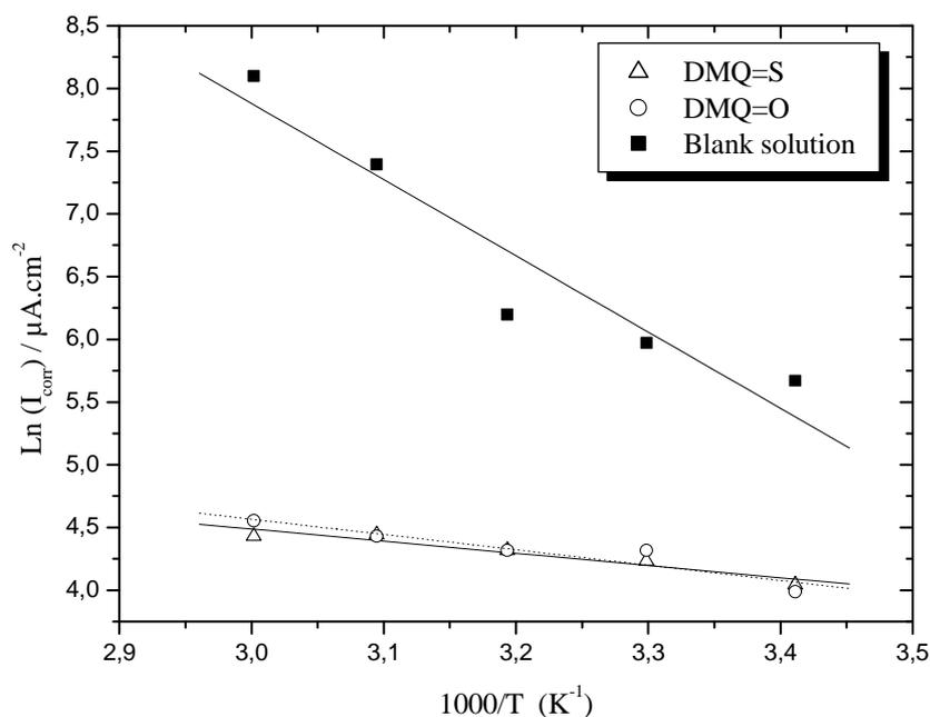
**Figure 6:** Relation between corrosion rate and reciprocal of temperature with and without inhibitors
