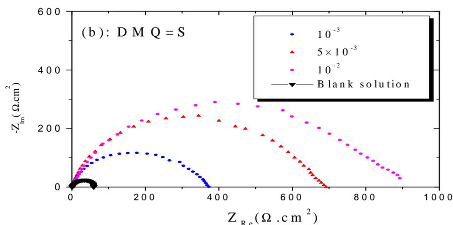
Figure 5: Nyquist diagrams for mild steel in 1M HCl at different concentrations of DMQ=S.
