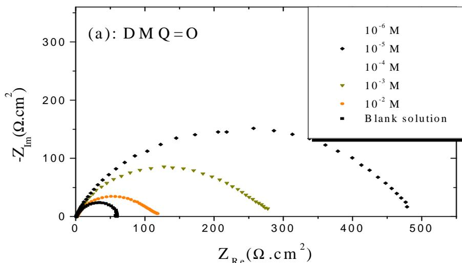
Figure 4: Nyquist diagrams for mild steel in 1M HCl at different concentrations of DMQ=O.
